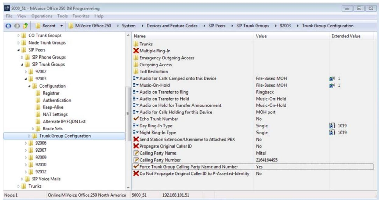
**Figure 7 – Example of Trunk Group Configuration**
