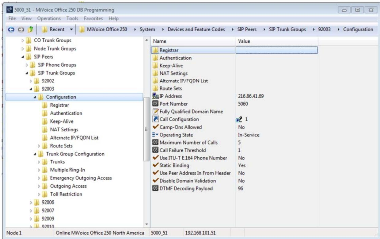
Figure 4 – Example of Configuration
