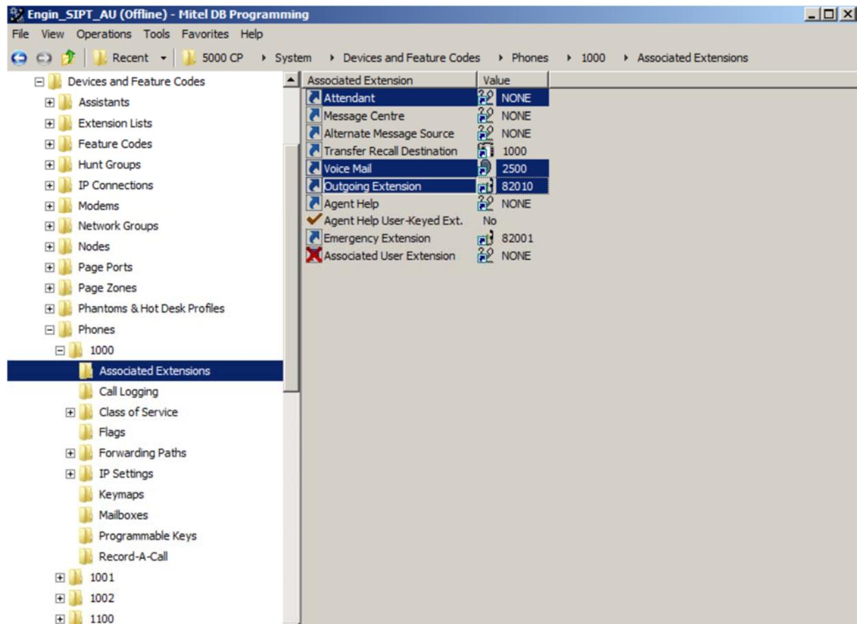
**Figure 9 – Configure outgoing extension for the phone**
